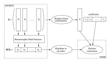
Fig. 1. On-the-fly Byzantine fault detection.
