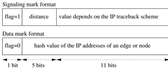
**Figure 4. Mark format for signaling and data subchannels**
