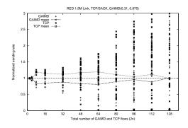
Figure 19. Normalized sending rates for 1.5Mbps RED link with TCP SACK
