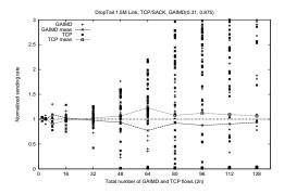
Figure 17. Normalized sending rates for 1.5Mbps drop-tail link with TCP SACK
