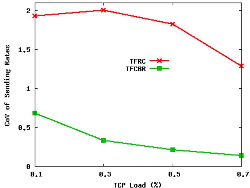
Coefficient of Variation (CoV) of TFRC and TFCBR in an interval of 1 minute when TCP load is 10% to 70% of the bottleneck link capacity.
