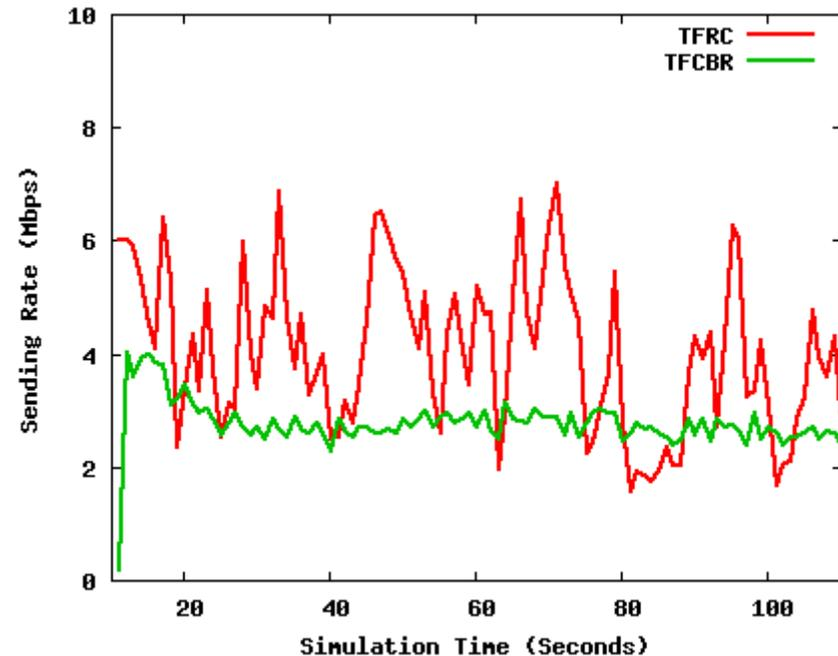
One-second average rate of TFRC and TFCBR when TCP load is 30% of the bottleneck link capacity.
