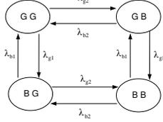
Fig. 9. Markov chain model for two independent fading channels.
