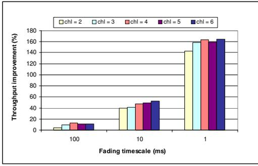
Fig. 19. Multi-channel diversity gains against fading timescale as the number of channels increases.
