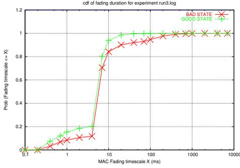
Fig. 2. cdf of MAC fading timescale: fast fading.
