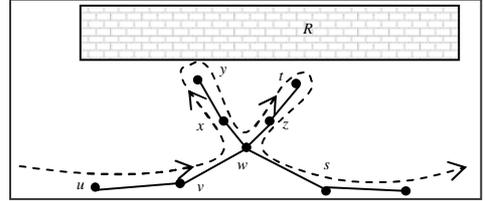
Figure 10 VSF traversal: VSF node  $w$  transmits more than twice
