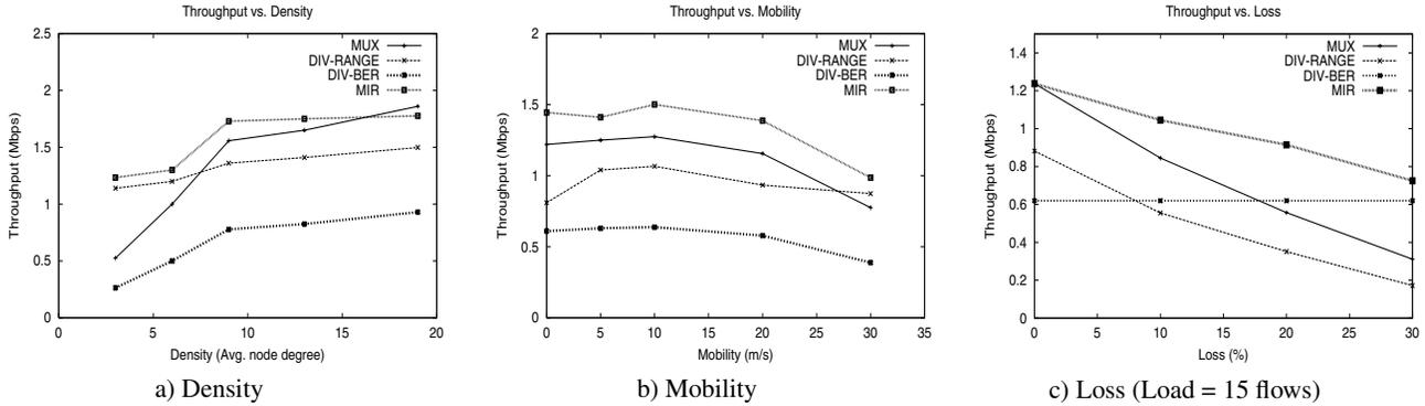
**Figure 3. Individual Impact of Components on Aggregate Throughput**
